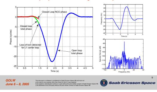
· Pulse shaped phase modulation generated by the simulator
